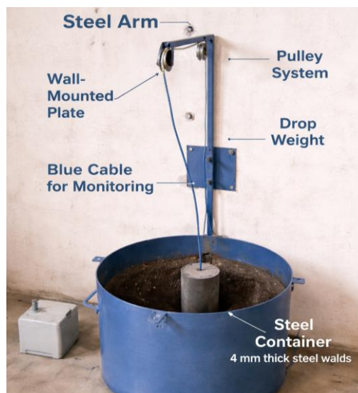
Figure 2. A steel arm is used in dynamic compaction to drop the weight
