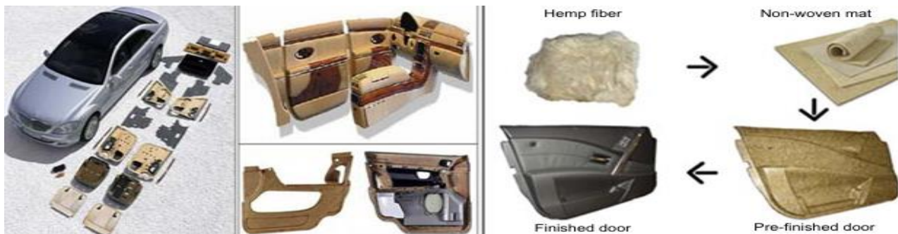
Figure 1. Automobile mechanisms founded on polymer composites reinforced with lignocellulosic fibers [6]
