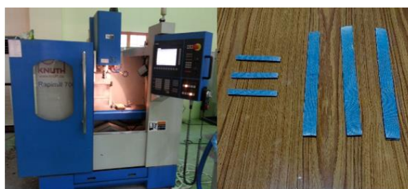
Figure 3. The CNC cutting machine (Rapimill 700 ) and the specimens
