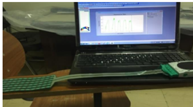
Figure 5. F-socket sensor measuring the interface pressure and connecting to a patient
