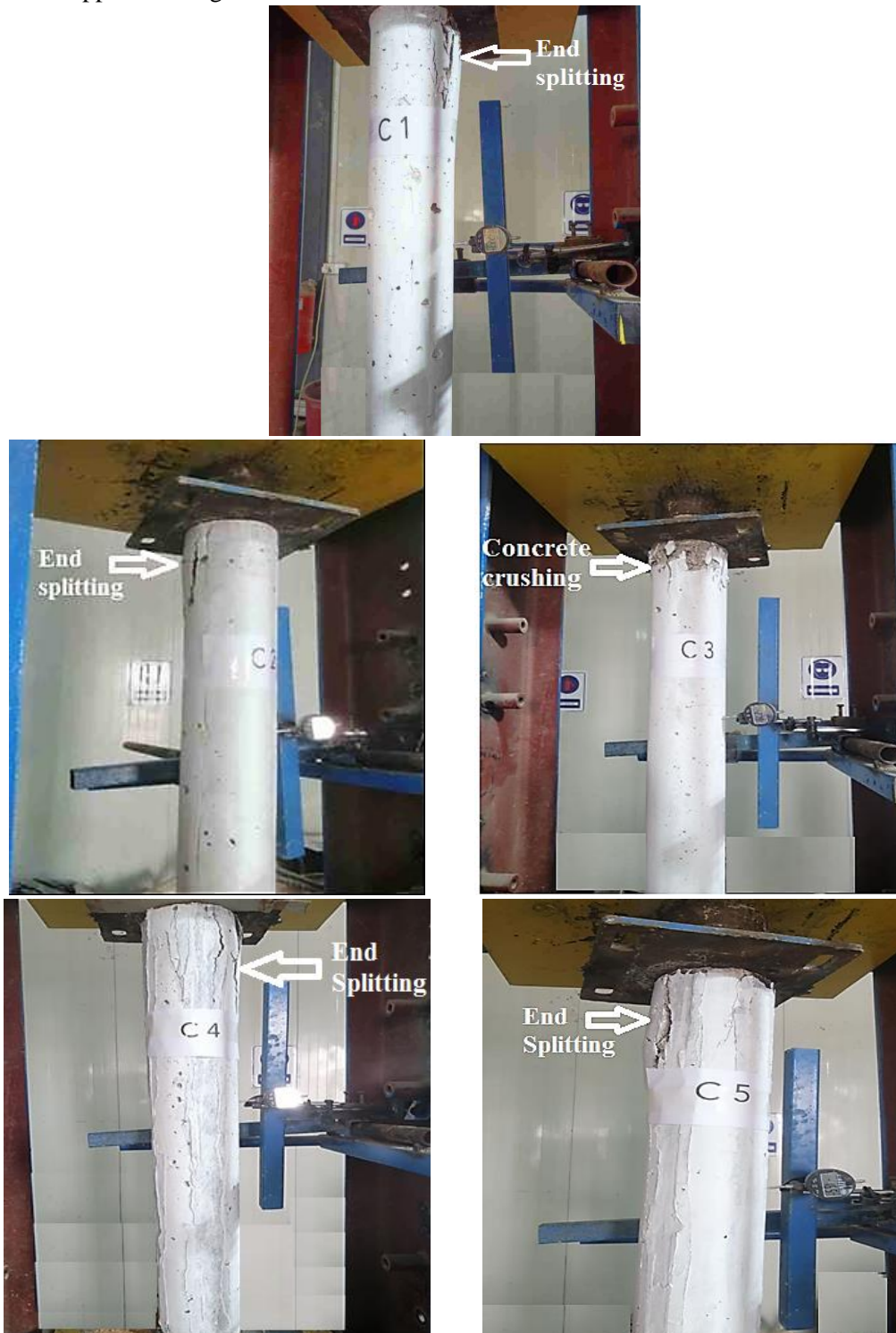
Figure 3. Crack patterns (C1-C5)
