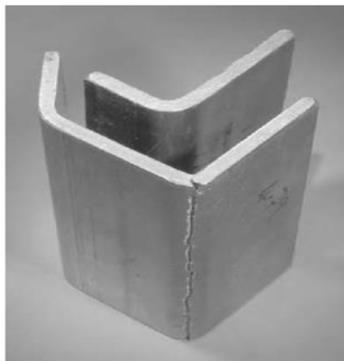
Figure 5. Performing bending tests on aluminum vehicle body panels [1]
