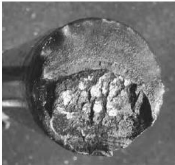
Figure 3. Fatigue failure of a machine's drive shaft (diameter = 25.4 mm) [1]
