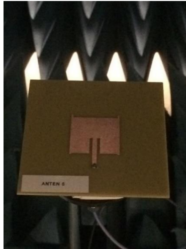
Figure 6. Fabricated antenna inside anechoic chamber
