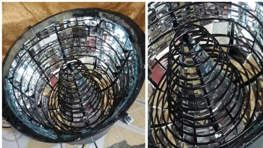
Figure 6. The installation of reflective mirrors and copper pipes with matte black paint
