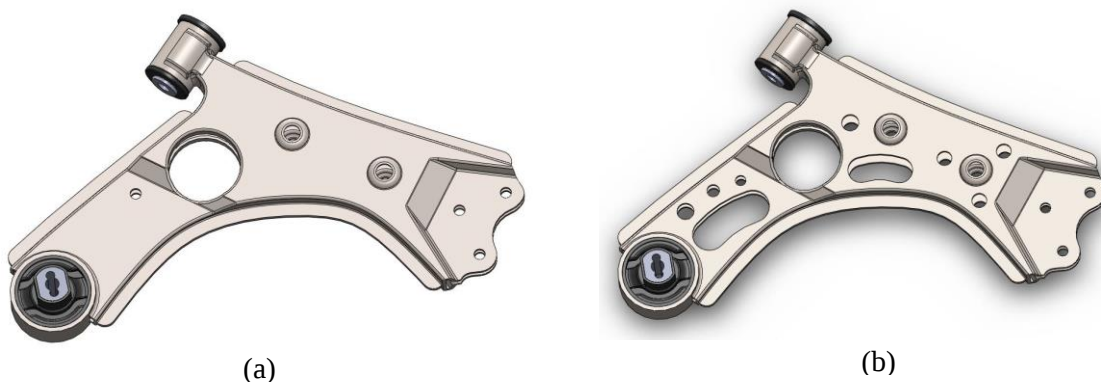
Figure 6. Lower suspension arm models a) first model b) final model obtained after topology optimization
