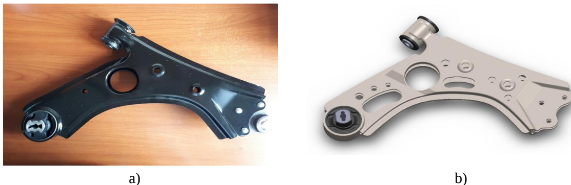
Figure 8. Lower suspension arm design, a) Before optimization, b) After topology optimization
