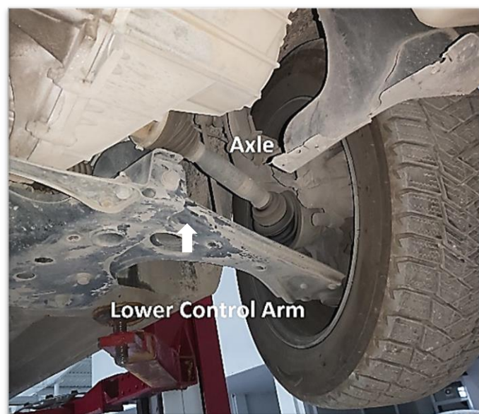
Figure 2. Lower suspension arm, axle, spring, and front wheel connection
